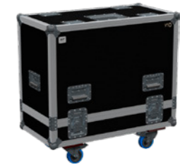
FC-V10 Flight-case for 2 x V10; 9mm birch multiplex, 4x100mm wheels, four big collapsible handles, 1 Label tour.
