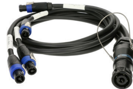
TYSP-NL8 Loudspeaker Y-Split set cable In NLT8MX, out 4 x NL4FC; cable 2 x 2.5mm 2 length 1m, 1,5m, 2m, 2,5m
