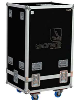
FC-CLa208 Flight-case for 4 x CLa208; PVC laminated 9mm birch multiplex, 4x100mm wheels, eight big collapsible handles, 1 Label tour
