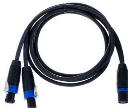
TYSP-NL4 Loudspeaker Y-Split set cable In NLT4MX, out 2 x NL4FC; cable 2 x 4mm 2 length 1m & 1,5m
